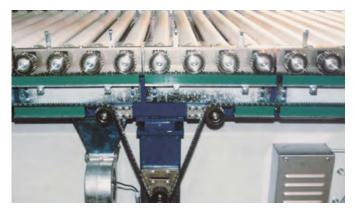
**Driving long roller tables with Biflex** During the annealing process for glass sheets in the roller hearth furnace, uniform synchronous running is critical. Slip-free drive system with Biflex inverted tooth chains. No backlash during reversing with two motors based on the master-slave principle.
