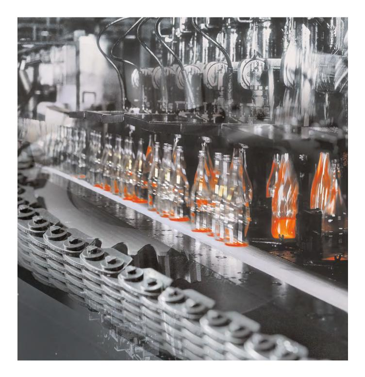
Safe, robust, and efficient. The glass industry is demanding. Drive and transport solutions not only need to reliably master operating processes, they also need to be highly resistant to harsh conditions and incredibly efficient. Inverted tooth chains cover all these requirements. They offer precise running characteristics, guarantee a long service life, and enable layouts optimized for specific applications with the utmost efficiency. And they have no qualms when it comes to high temperatures.
