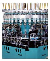
*Medical glassware A single Biflex inverted tooth chain is used for the synchronous rotation of all 32 forms in a forming glass lathe for processing glass vials.*
