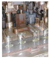
*Special version for small glass products Individually adapted inverted tooth conveyor chains for a flask production line.*
