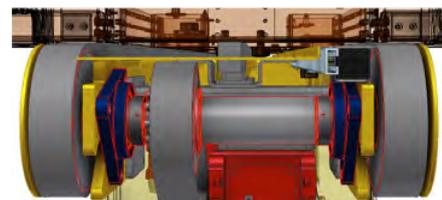
Head drive on a chain conveyor (housing hidden from view)
