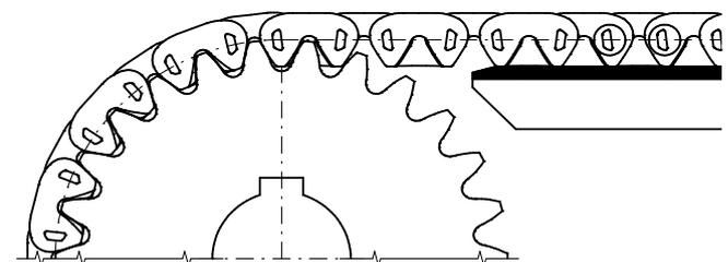
*Inverted tooth chain on sliding material*
