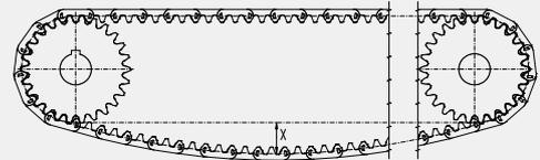
b) If the slack span is supported in the profile
