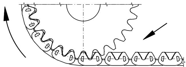
*Lubrication should always be applied on the tooth side*
