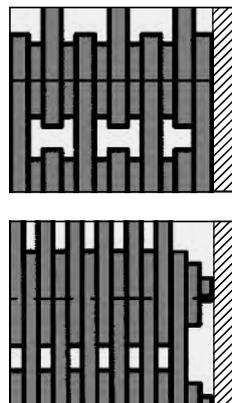
Rolling pivots are laser-welded in the outer plates of inverted tooth conveyor chains from Renold. The rivet heads no longer protrude and the inverted tooth chains can be placed flush to the sides with minimal gapping. This increases the operational reliability and safety of the chain and the chain width remains constant throughout its entire service life.
